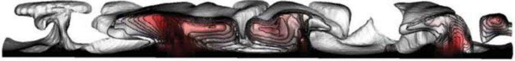
FIGURE 1. Hot plumes visualized with 20 isotherms for T \in [0, 0.5] in a subdomain of width 0.2R , DNS for Ra = 10^5 , Pr = 0.7 , \Gamma = 10 .
